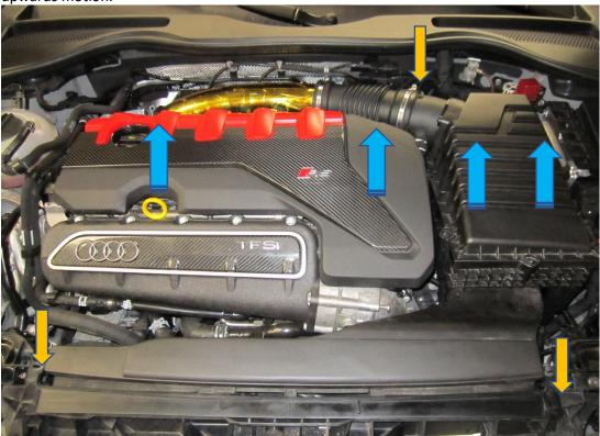
2. Unplug the MAP sensor, TPS sensor and t30 torx that hold the rocker cover bracket and the stock dumpvalve, then undo the hose clamp that holds the boost hose to the cast elbow.
