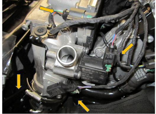
3. Remove three of the four t30 torx fasteners that hold the cast elbow to the throttle body and inlet manifold, Then undo the five M10 bolts that hold the inlet manifold together.
